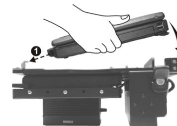
5. Pull the expansion bus connector latch all the way outward (1) and at the same time use the included key to lock the latch (2) in order to secure the computer to the vehicle docking.
