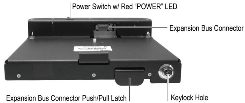
The red LED light, built into the power switch, indicates that there is power to the unit.
